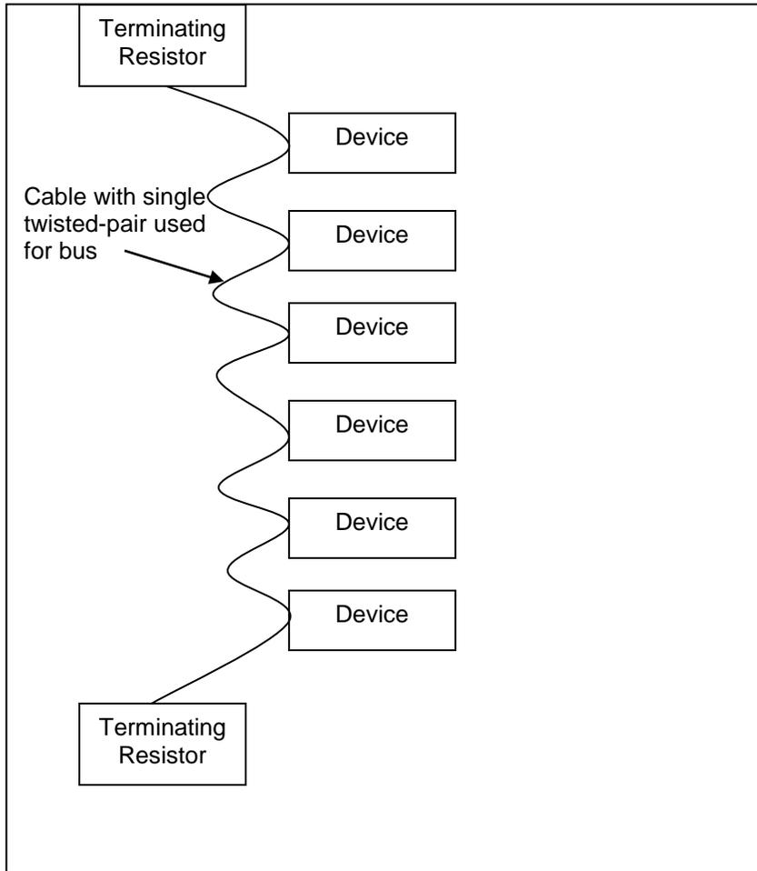
**Fig. 2 Conventional Active HUB RS-485 wiring**
