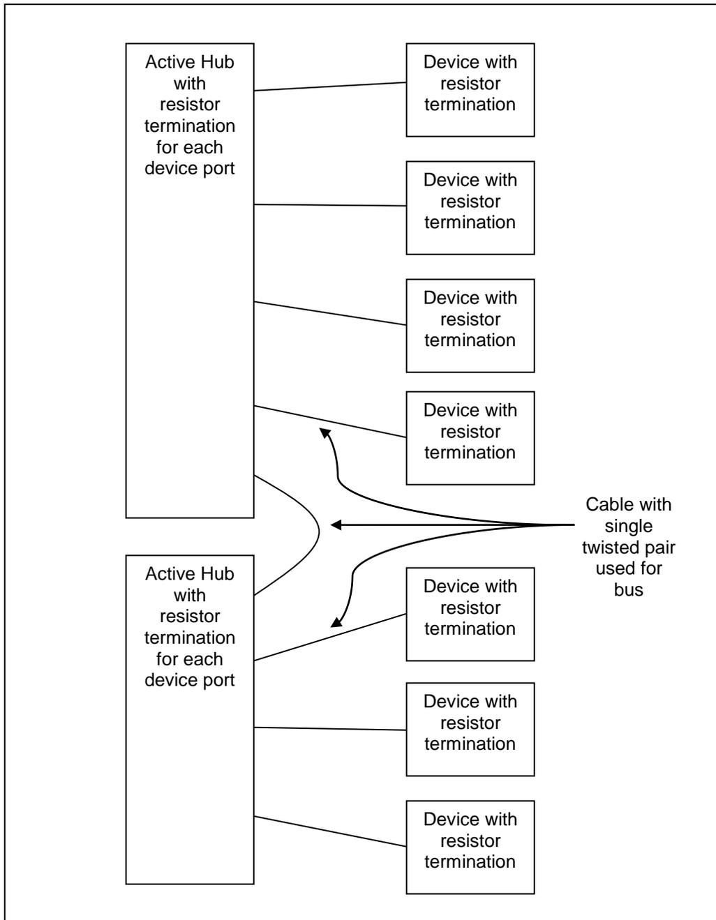
**Fig. 3 “Folded Daisy-Chain” Passive Repeater Hub**
