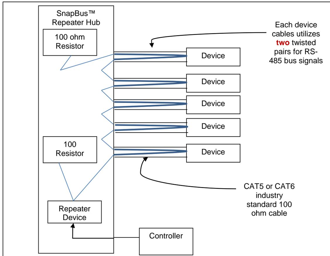
**Fig. 4** Folded-Daisy-Chain RS-485 wiring showing a device connection using two terminals.
