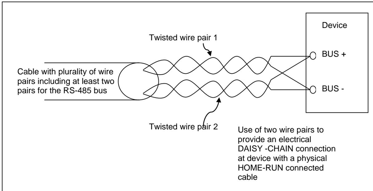
**Fig. 5** Folded-Daisy-Chain RS-485 wiring showing a device connection with four connection terminals. The SnapBus system connector can be built into the Device as shown:
